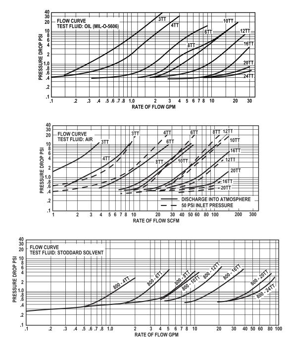
Note: Pressure drop curves are based on approximately 8" H<sub>2</sub>O cracking pressure. Where lower (special) cracking pressure is used, pressure drop will be lower in the low flow rate range.
