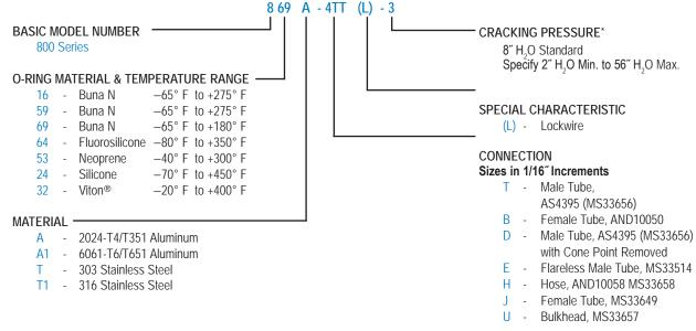
\* NOTE: For cracking pressure less than 8"  $H_2O$ , cracking pressure tolerance is Max.; for higher cracking pressure, cracking pressure tolerance is  $\pm 10\%$  with gas, or +15 -40% with jet fuels. Cracking pressures over 56"  $H_2O$  should not be specified without consulting factory.
