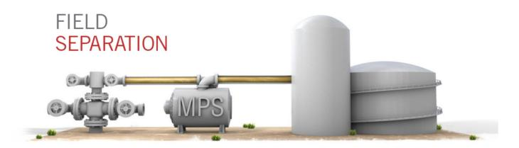
In field separation, the wellhead facility exerts a required pressure on the well to drive the production fluid through a local separation/ takeaway processing battery.
